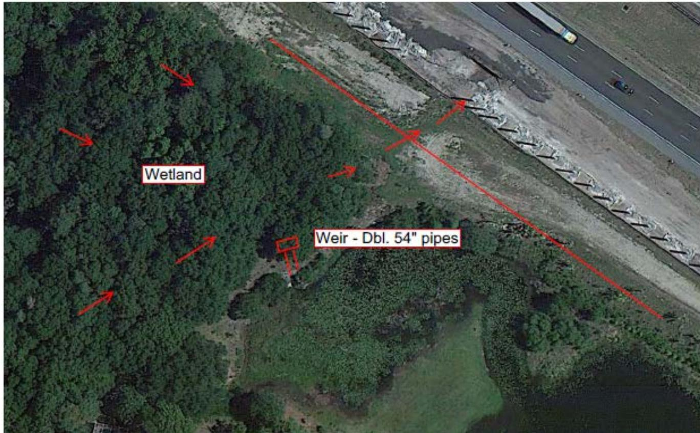
Prepared By FDOT August 2012 This Schematic Depicts Watershed Flow From TPOST 3 Under I 75 – In Direction of Trout Creek
